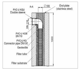
The end pieces of the DRAINFIX CLEAN channel with the lateral discharge outlets must always be installed at the lower end of the respective channel run, in order to avoid water pooling in the filter substrate. Optionally it is possible to fit additional end caps at channel section ends. This ensures that section ends can be recognised from the outside after backfilling the excavation with filter substrate.
